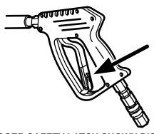
TRIGGER SAFETY LATCH SHOWN DISEN-GAGED Figure 2 \_\_\_\_\_
